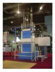
processes the cut is performed in one pass of the broach, which makes it very efficient.
